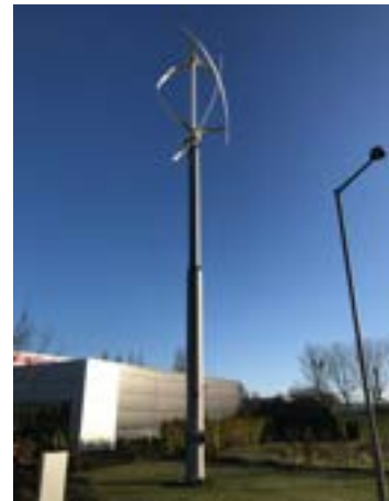
Figuur 8. Verticale as windmolen (bron: https://www.quietrevolution.com/ )
